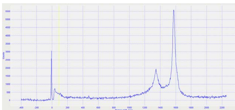
Fig. 2. Raman spectrum of the synthesized multi walled carbon nanotubes
